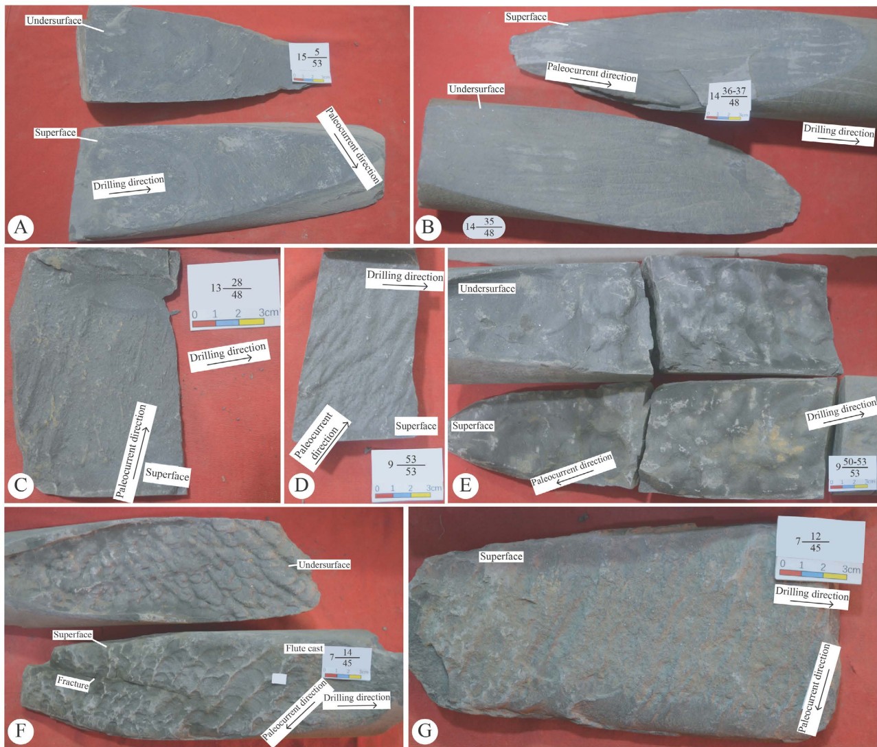
Figure 6. Bedding plane structures of Well Y core in Block X of Huaqing Oilfield, Ordos Basin. (A) Small-scale flute cast. 15-5/53. (B) Groove cast. 14-(36-37)/48. (C) Small-scale flute cast. 13-28/48. Superface. (D) Small-scale flute cast. 9-53/53, Superface. (E) Load cast. 9-(50-53)/53. (F) Large-scale flute cast. 7-14/45. (G) Small-scale flute cast. 7-12/45. Superface.
