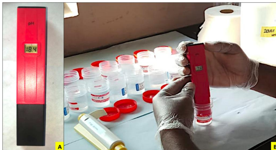
Fig. 2. This image shows the estimation of salivary pH. (A) - Digital pH meter (Pen type pH meter). (B) - pH meter used for estimation of pH from the sample
