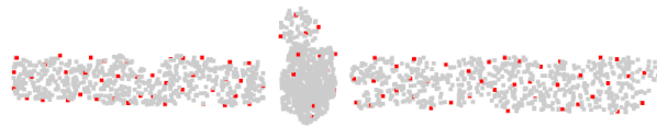
Figure 11. The ISS keypoint extraction result. The red points are the selected ISS keypoints.
