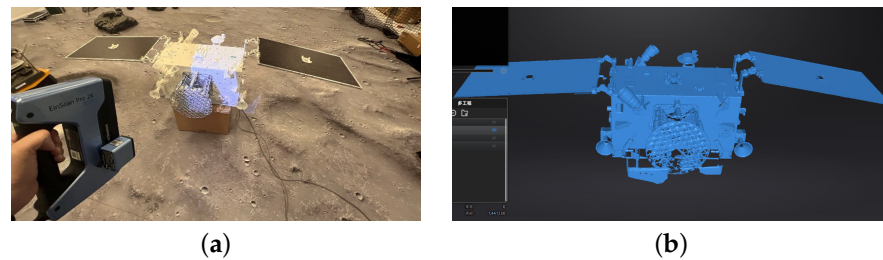
Figure 6. 3D scan system: (a) 3D scanner scan spacecraft. (b) 3D scan point clouds.
