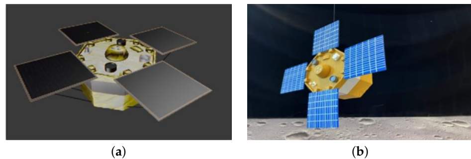
Figure 2. The CAD model and 3D printed model of ArcimSAT: (a) CAD model. (b) 3D printed model.
