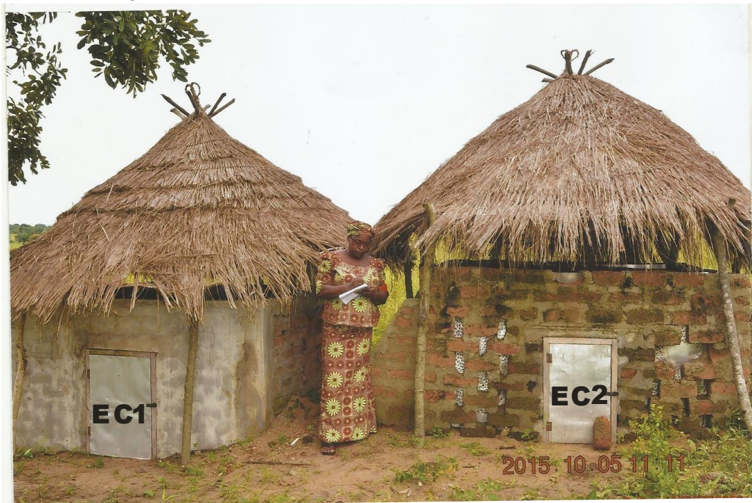
Plate 1. Evaporative coolers 1 & 2 EC1= Non-Cladded Burnt-Clay-Brick Evaporative Cooler (NBBEC) EC2=Aluminum-Cladded Burnt-Clay-Brick Evaporative Cooler (ABBEC)
