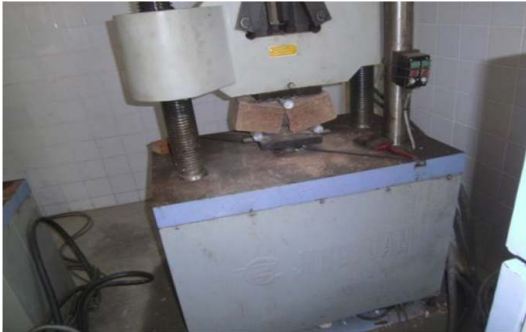
Fig. 3. Test of resistance in inflexion (three points) on CEB
