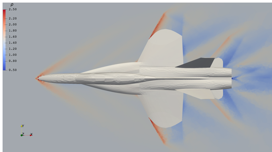
Figure 26. Comparison between the third-order solution (upper half) and the first-order solution (lower half) of Problem 6 on the z = 0 surface (top view).
